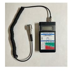
**2. Bearings:** properly maintained bearings allow the mill to run smoothly. When bearings start to fail, there will be excessive temperature & mill vibration. All factory assembled rotors leave our facility vibration free. When the vibration analysis exceeds 0.9 millimeters per second, it is time to prepare for system shut down and replace the bearings.
